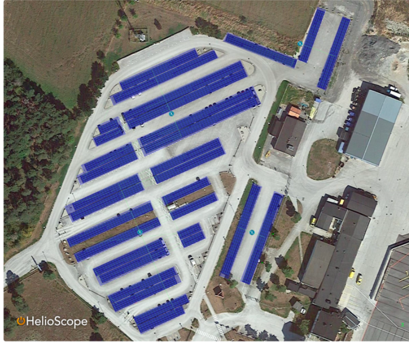
Figure 3: Modeled PV array location (marked as blue sections) at Visby Airport used in scenario analyses.
